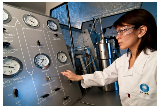
The triaxial stress rig is used for integrated characterisation of coal permeability behaviour with effective stress and gas adsorption.
