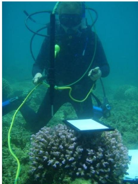
Figure 4. Diver collecting underwater spectra of coral using Ocean Optics spectrometer.
