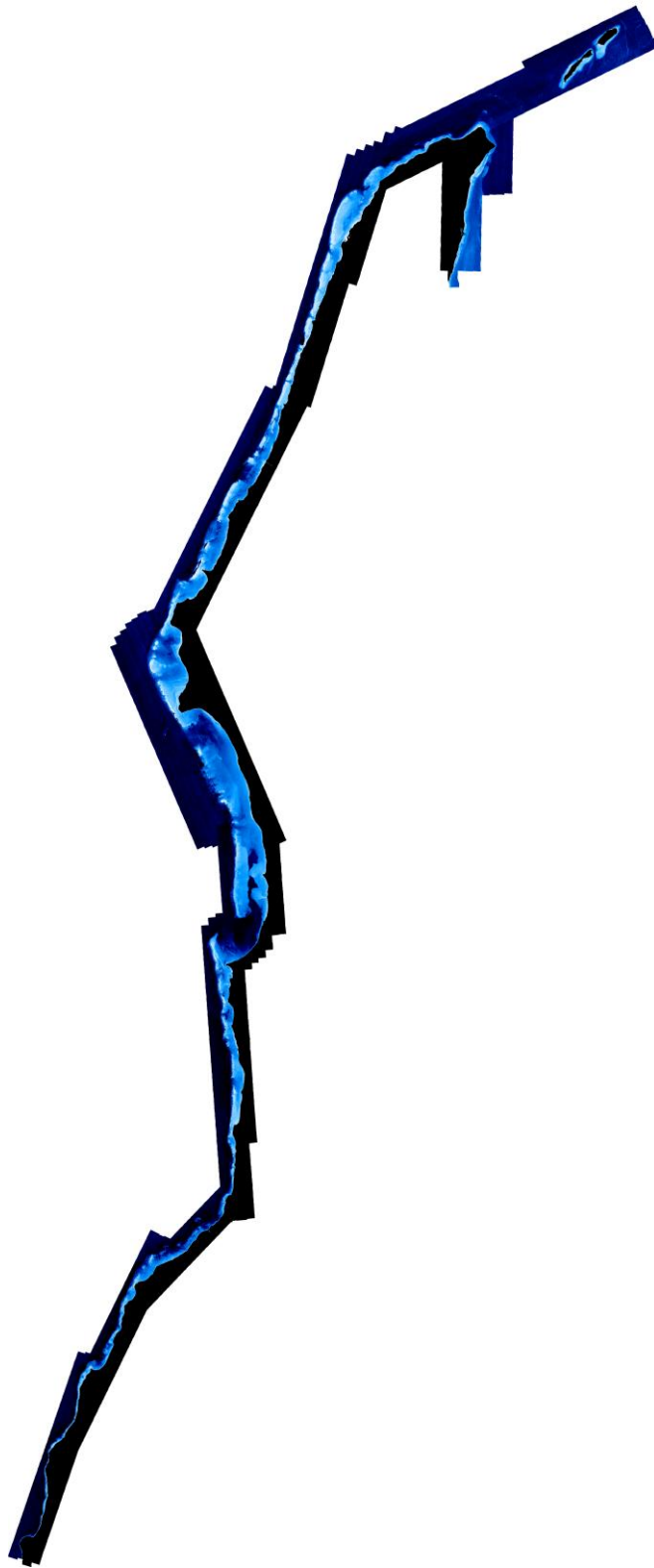
Figure 1: Hyperspectral image-derived bathymetry mosaic of the Ningaloo Marine Park. Depths range from 0 m (white/light blue) to 30 m (dark blue). The land mask on the RHS of the imagery is shown as black.
