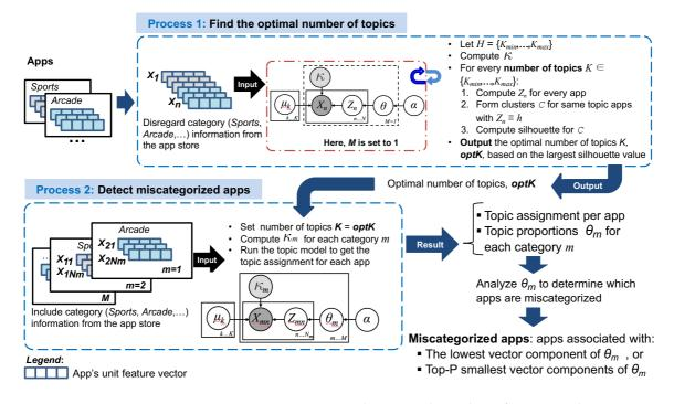
Fig. 4: Two main processes in FRAC+: **Process 1**. Detect the optimal number of topics and **Process 2**. Detect miscategorization - which is achieved by running again the topic model using the optimal number of topics from Process 1 and the app category information. See text for details.
