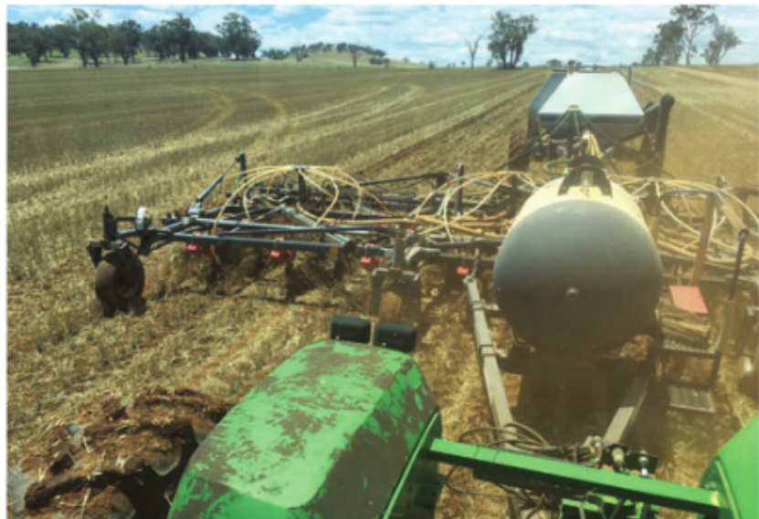
A DRIVER'S-SEAT VIEW OF STUART'S DISC SEEDING RIG HE EXPECTS TO MAKE IT EASIER FOR HIM TO SOW ACCURATELY THROUGH THE HIGH RESIDUE LOADS HE AIMS TO RETAIN TO PROTECT AND FEED THE SOIL.
