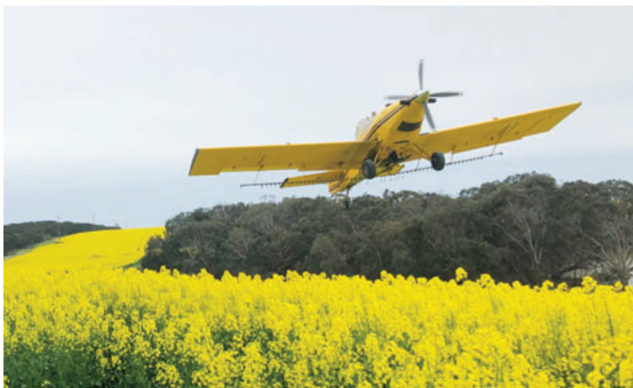
THE PONTIFEX FAMILY’S AIR TRACTOR IN ACTION APPLYING A CHEMICAL TO A CROP OF CANOLA.
