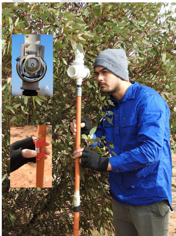
Figure 2.1. Cover survey staff with densimeter (A) and laser pointer (B) attached to a graduated staff (TERN image)
