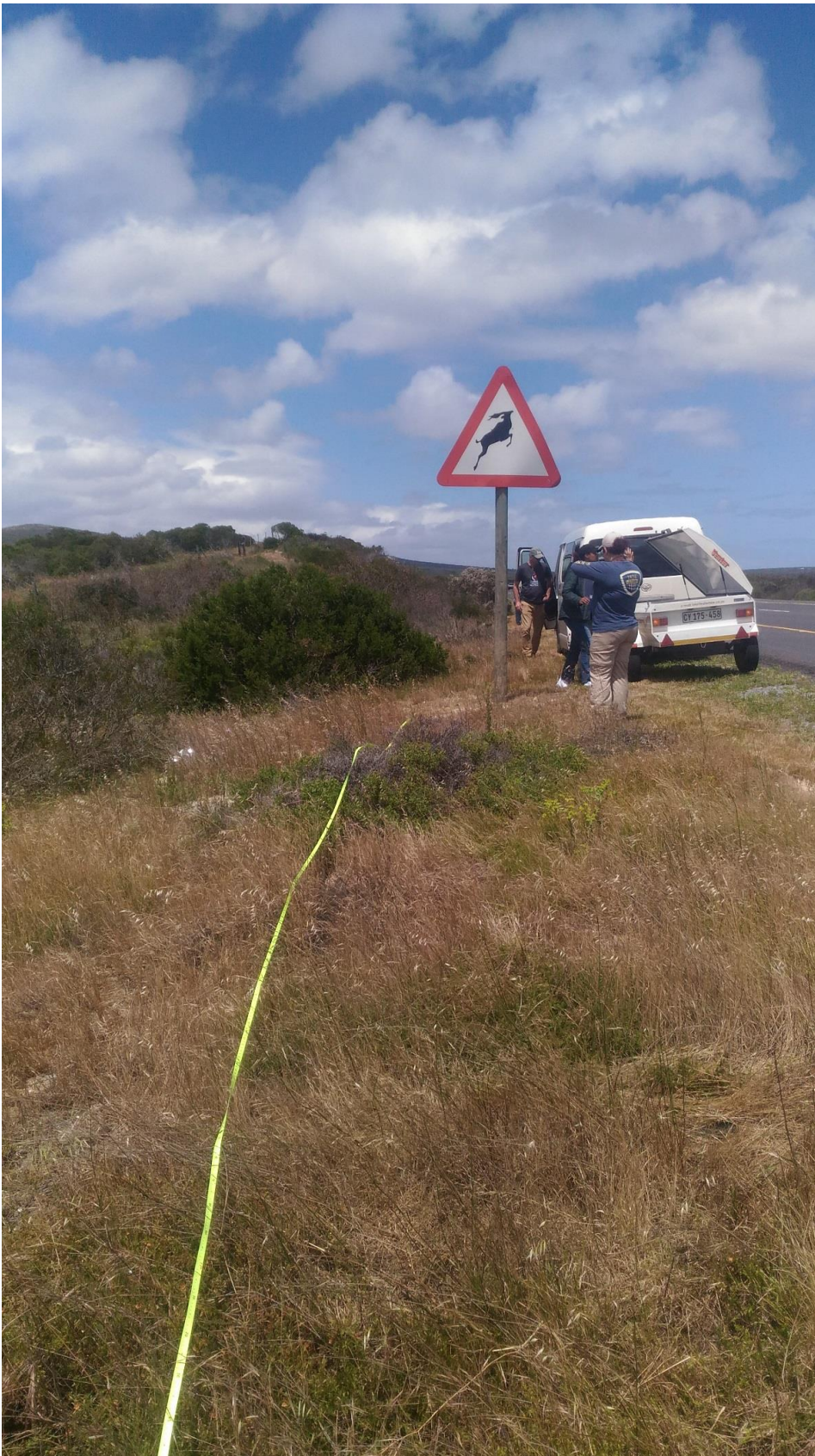
Figure 3.7 Transect method of debris survey at an inland (rural) survey site
