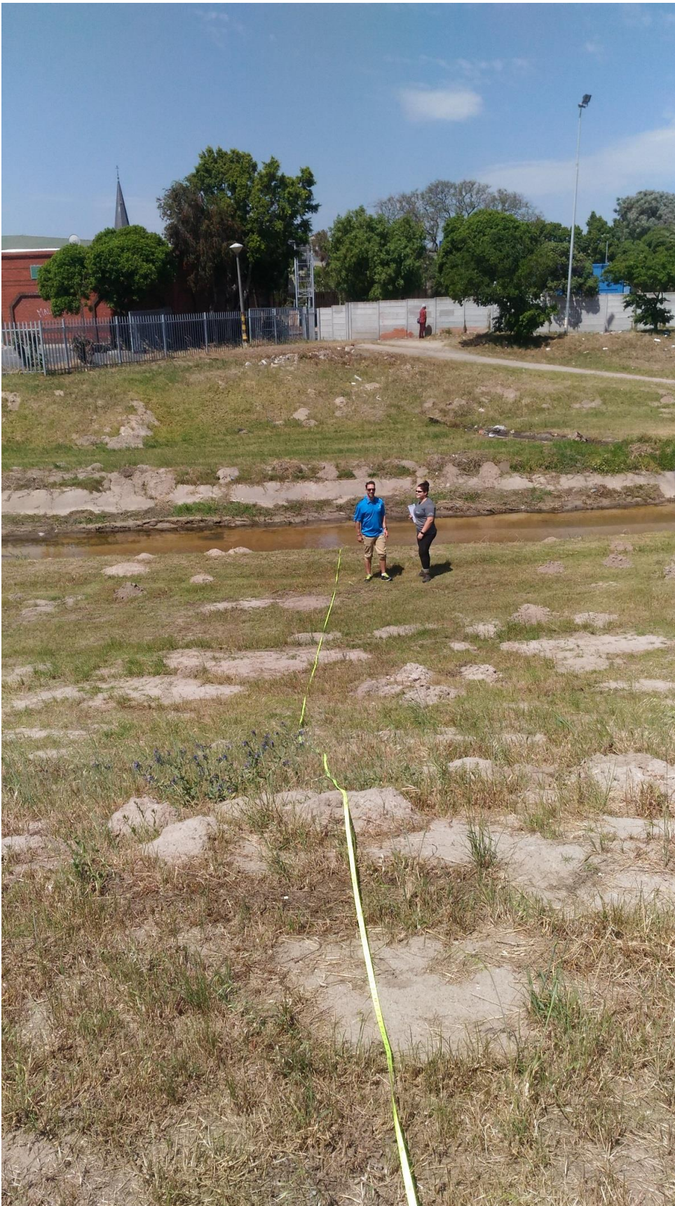
Figure 3.9 Example of river survey being conducted from the water's edge to the top of a flat riverbank.
