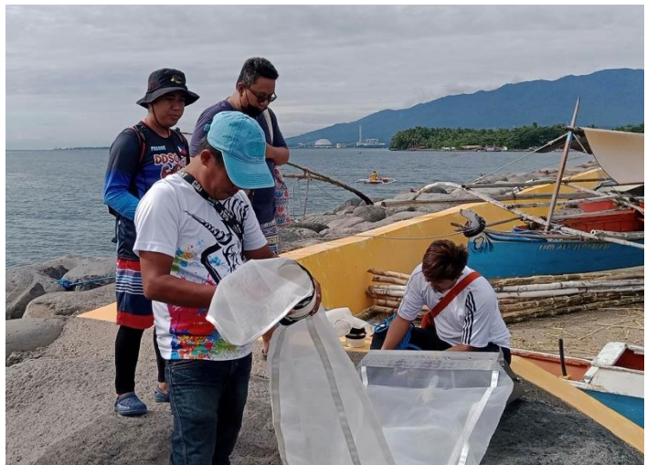
Preparing a standardised manta tow net used for sea surface trawl sampling.
