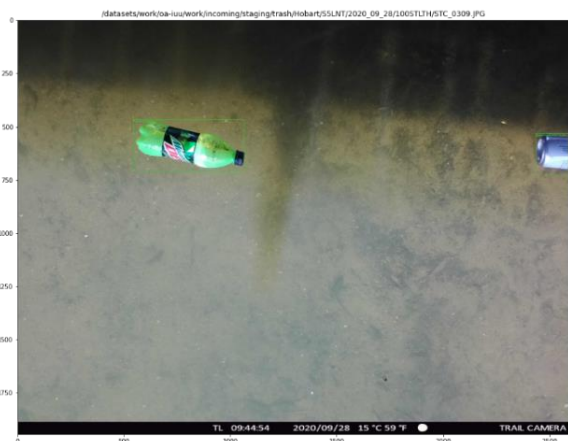
Figure 3: Example of litter detection and classification by our system in waterways.
