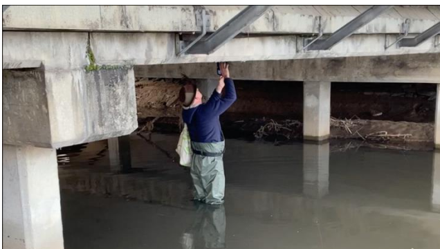
Chris Wilcox setting up a trail camera to monitor litter flux in a stormwater drain in Hobart.
