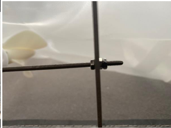
Figure 4.9 Position of nuts on net frame
