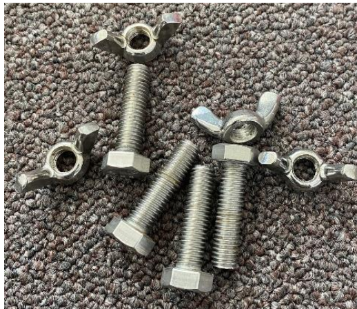
Figure 4.3 Screws and wingnuts to hold the sides of the frame
