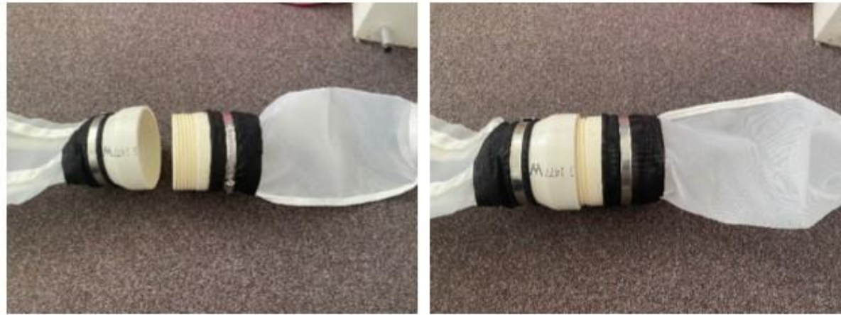
Figure 4.5 Screw the cod end onto the net
