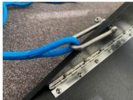
Figure 4.11 Attach the two ends of the rope to the two D shackles
