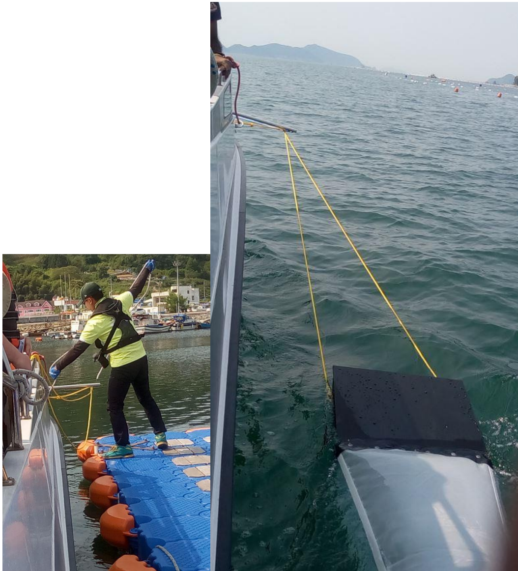
Figure 4.2 A surface trawl net towed by a boom on the side of a boat, note the net should run parallel with the boat and the ropes should not be twisted. The black top wood structure of the net should skim along the surface of the water.
