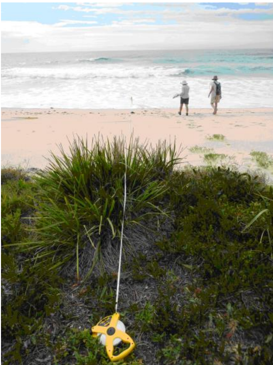
Figure 4.5 The survey transect should run 2m into backshore vegetation
