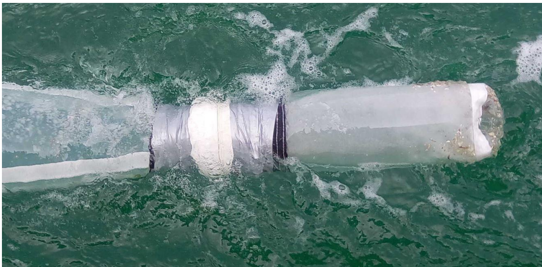
Figure 4.6 Cod end on net as it is being towed. Note the duct tape around the clip holding mesh on to pipe, not necessary but is a good precaution
