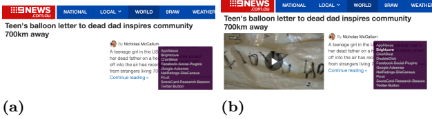
Fig. 8. Ghostery's filters (a) video content by blocking brightcove widget on www.9news.com.au . Once unblocked, brightcove loads (b) video content on the web-page.
