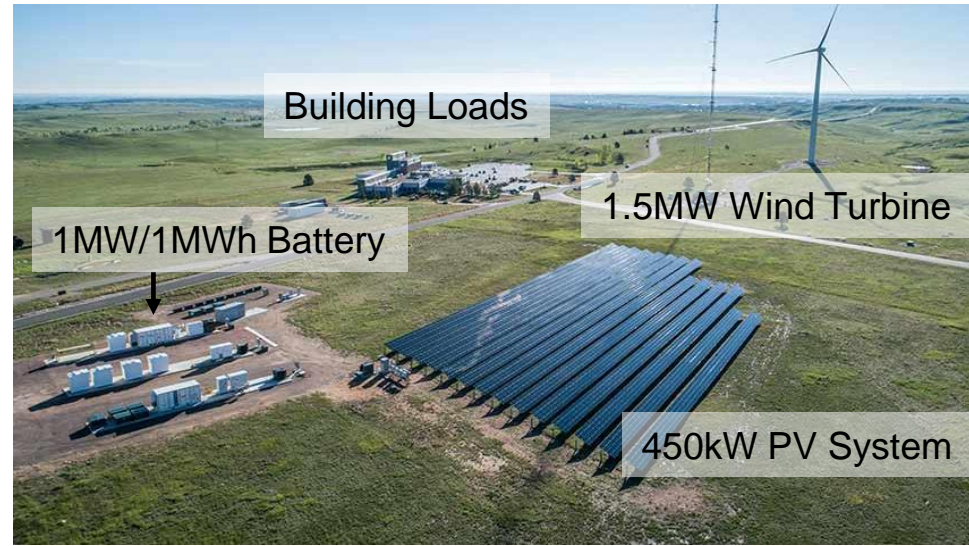
24-hour operation of Wind-PV-Battery System at NREL's Flatiron Campus
