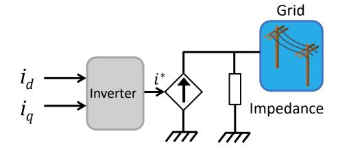
Control **output current** based on desired output power (active and reactive)
