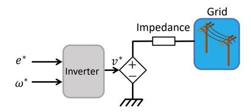
Control **PWM voltage/angle** based on desired output power (active and reactive)
