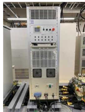
GFM/GFL inverter prototype with synthetic inertia capability
