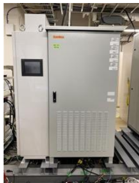
GFM/GFL inverter prototype with synthetic inertia capability
