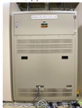
GFM/GFL inverter prototype with synthetic inertia capability
