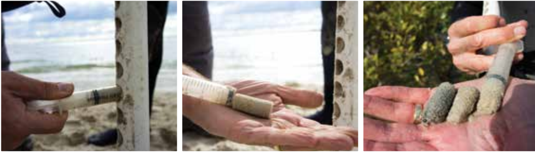
Figure 3.12 Cores are collected using a corer with predrilled sampling ports and sub-cores removed using cut-off polyethylene syringes (© Sarah Hoyt, CI).
