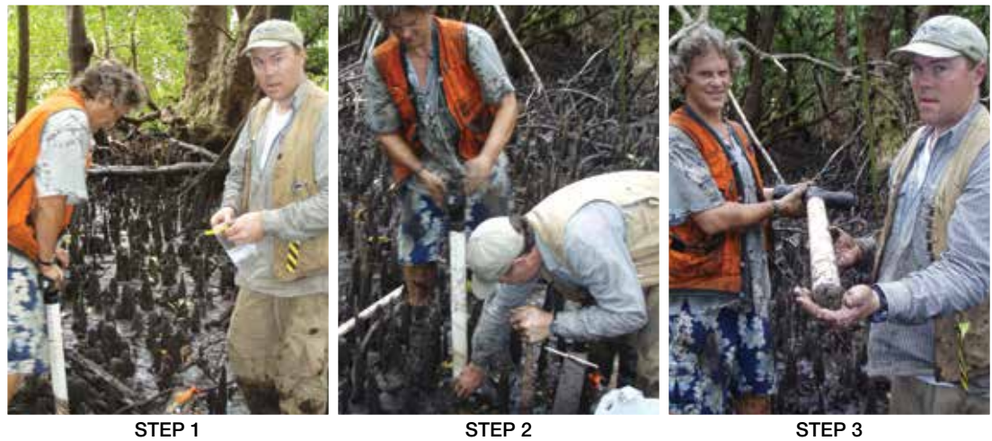
Figure 3.5 Sampling a soil core using a soil auger (© Boone Kauffman, OSU)
