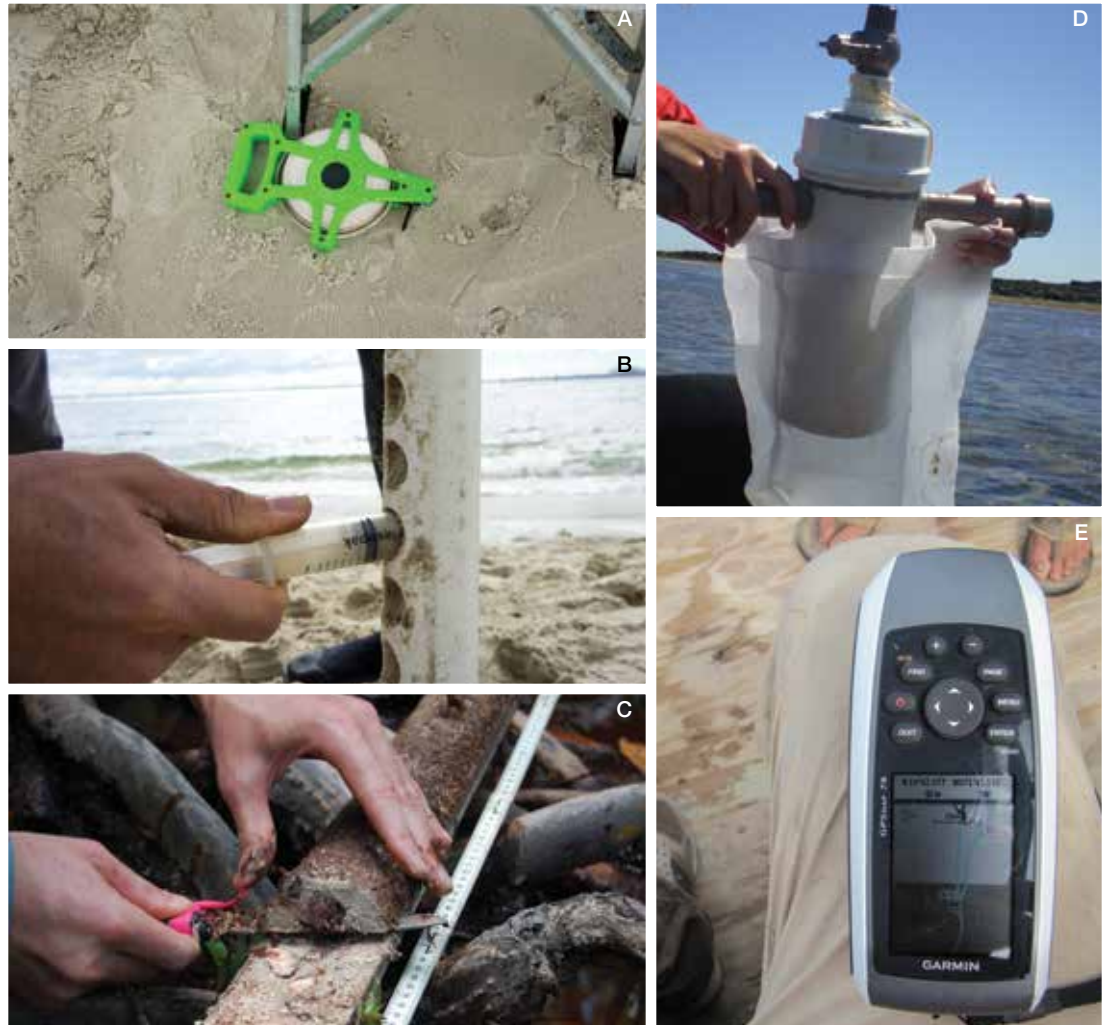
Figure 3.3 Equipment typically needed for field collections of soil carbon. (A) Measuring tape for measuring depth along the soil core (© Sarah Hoyt, CI), (B) Syringe used to subsample core (© Sarah Hoyt, CI), (C) Knife used for subsampling (© Boone Kauffman, OSU), (D) Core & sample bag (© Krishna Barros, UFC), and (E) GPS to mark coring position (© Boone Kauffman, OSU)
