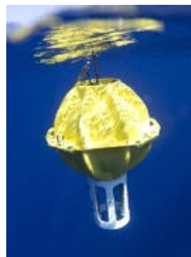
Deep APEX (below left) and Deep SOLO (below center) 6000 m floats. Location of 13 active Deep SOLO (blue) and Deep APEX (red) floats (below right) in the SW Pacific Basin
