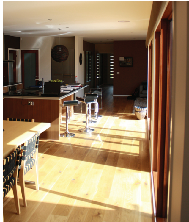
FIGURE 4 North-facing glazing allows winter sun into the building. (Michael Ambrose)
