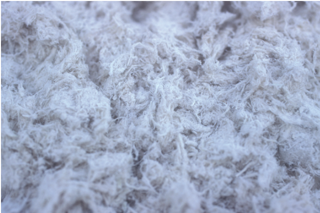
FIGURE 5 Asbestos fibres – seen here in sprayed asbestos insulation – have a shaggy appearance. (Stock.com/Brasil2)
