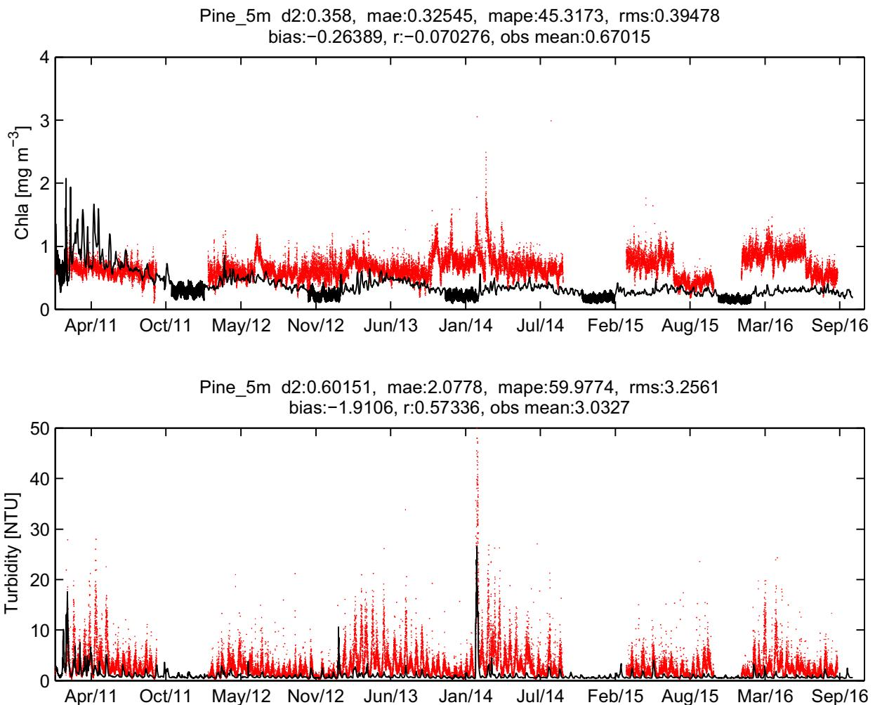
Figure 54: Pine Island Mooring Marine Monitoring Program (MMP) observations against GBR4 model: Observation (blue), model (black): Parameter/s = Turbidity and Chlorophyll (fluorescence). Field observation depth taken: 5 m. Model grid deepest point at this site -18.14 m. Observation deepest point at this site 20.0 to 25.7 m.
