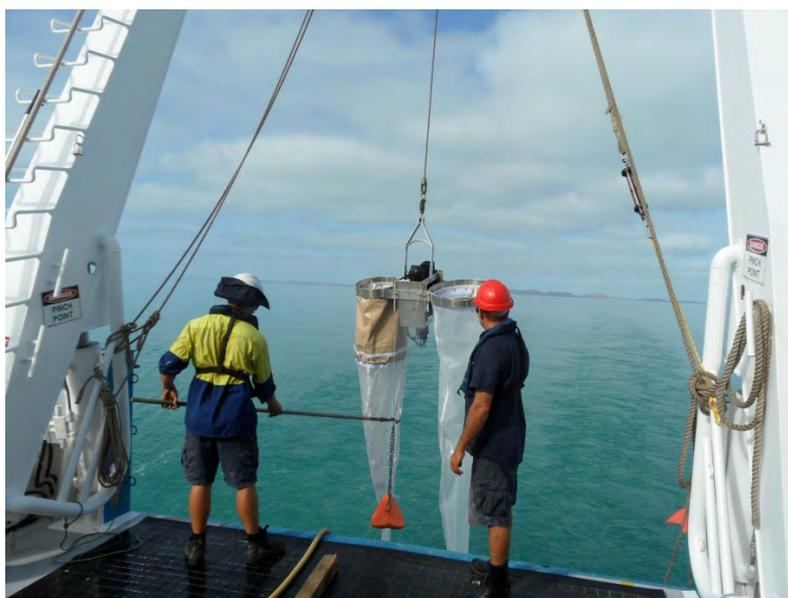
Figure 4.7.13. Size-fractionating bongo net. The net on the left comprises a 150 $\mu$ m mesh net nested within a 73 $\mu$ m mesh net; the net on the right is a 355 $\mu$ m mesh net. An instrument package sits between the two nets, and includes a Laser Optical Plankton Counter (LOPC) and CTD unit.
