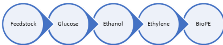
Figure 9 – Production of ethanol for bioPE manufacturing.
