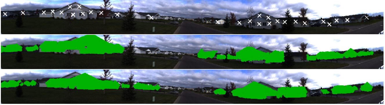
(a) Image 1: 2D features (top), building points projected using RANSAC camera pose (middle) and building points projected using our pose (bottom).
