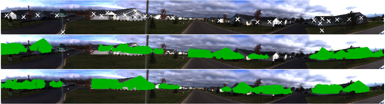
(a) Image 5: 2D features (top), building points projected using RANSAC camera pose (middle) and building points projected using our pose (bottom).
