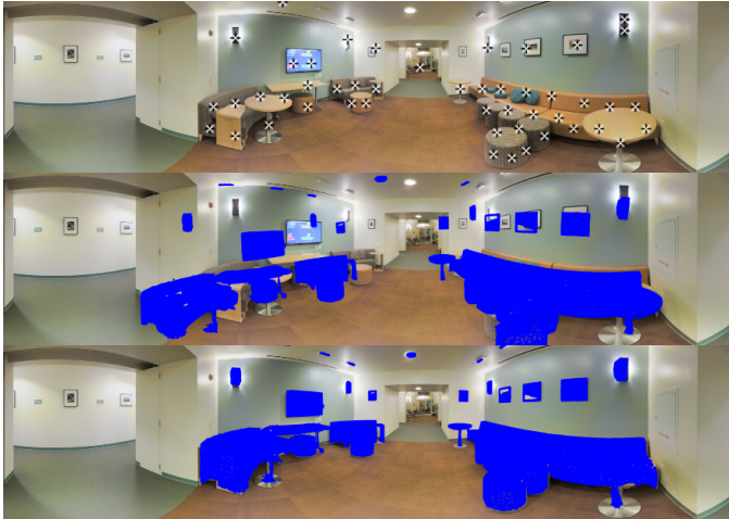
(b) Panoramic photograph and extracted 2D features (top), furniture points projected onto the image using the RANSAC camera pose (middle) and furniture points projected using the GOPAC camera pose (bottom).
