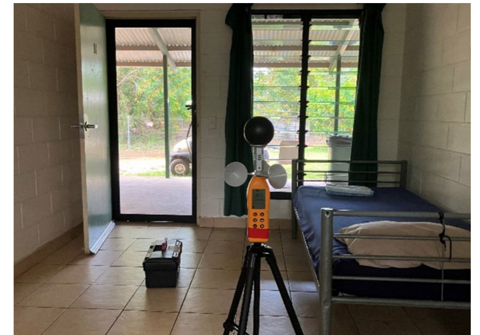
Figure 55. Two accommodation designs monitored in December 2023. Left: 'Village design', cement block walls of a light colour, uninsulated and unventilated roof with reflective foil (sarking), minimal shading by eaves with no eaves on the west and east orientations, ventilation provided by air bricks with little potential for cooling from cross breezes, and 450 mm mechanical wall-mounted fans. Right: 'Harmony design', cement block walls of a light colour, uninsulated and unventilated roof with reflective foil (sarking), rooms orientated to the north-west to capture prevailing breezes, large eaves providing shade, ventilation through louvre windows with 90% opening to the breeze, and ceiling fans.
