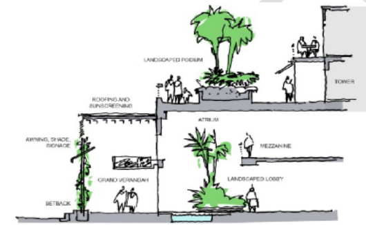
Figure SC6.16.3.8.d – Street canopy (typical cross section)
