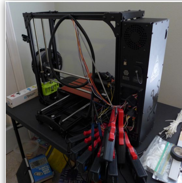
Figure 3: Our Lulzbot Taz 6 printer, instrumented by two PicoScope 5444D oscilloscopes. The probes are 60A Inductive Current Clamp probes, also by PicoScope. Each motor (highlighted) has two clamps attached, one for each phase. The fan controller is also instrumented by a standard voltage probe. The data captured here is transmitted to a host PC running the PicoScope application.
