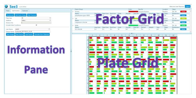
The **Information Pane** reads from and writes to the underlying database. This pane allows one to select the 'Plate Size' - the size of the optimisation: 24 well (4 rows x 6 columns); 48 well (6 rows x 8 columns) or most commonly 96 well (8 rows x 12 columns). Following standard convention, rows are lettered and columns are numbered and is always shown in portrait orientation with well A1 in the upper left hand corner. Thus a 96-well plate has rows A-H, columns 1-12.
