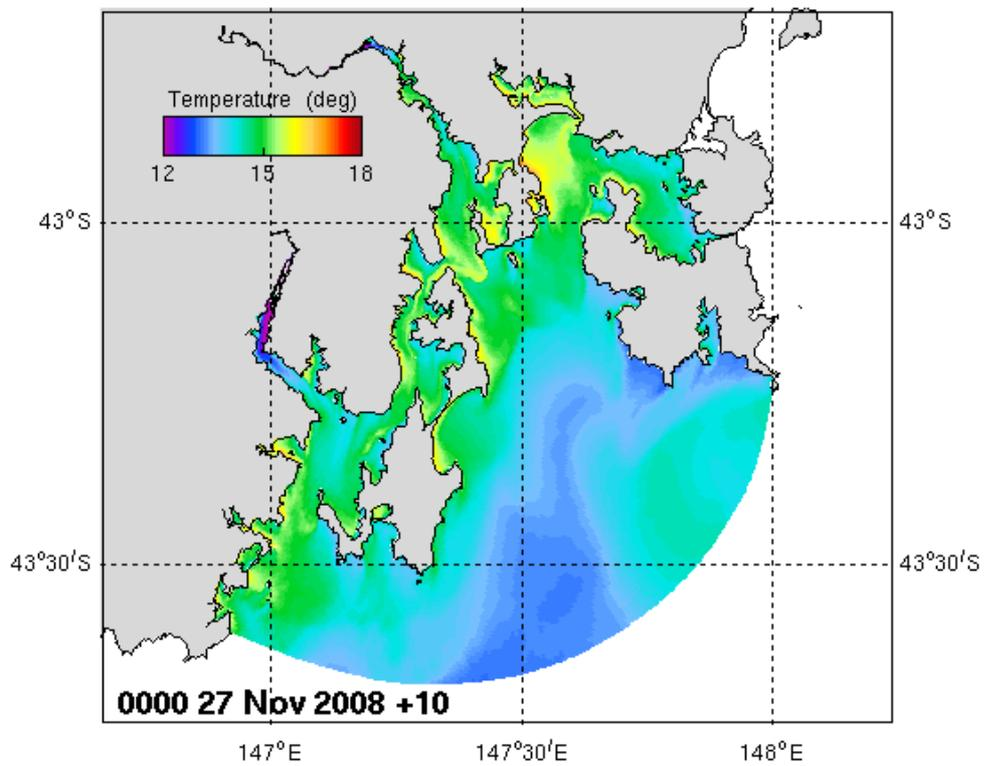
Figure 2.26. Surface temperature output from the STORM model.
