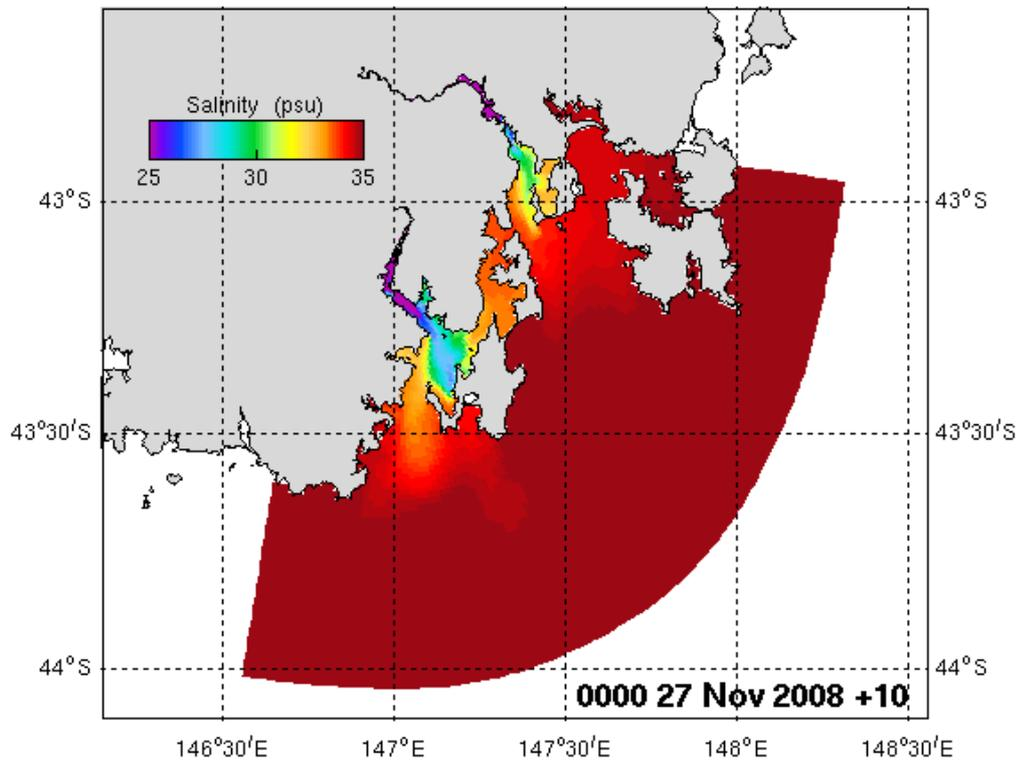
**Figure 2.27. Surface salinity output from the SETAS model.**
