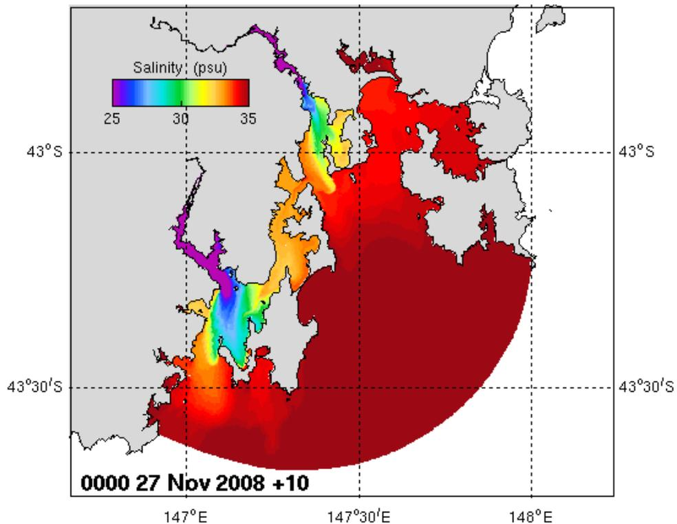
**Figure 2.28. Surface salinity output from the STORM model.**
