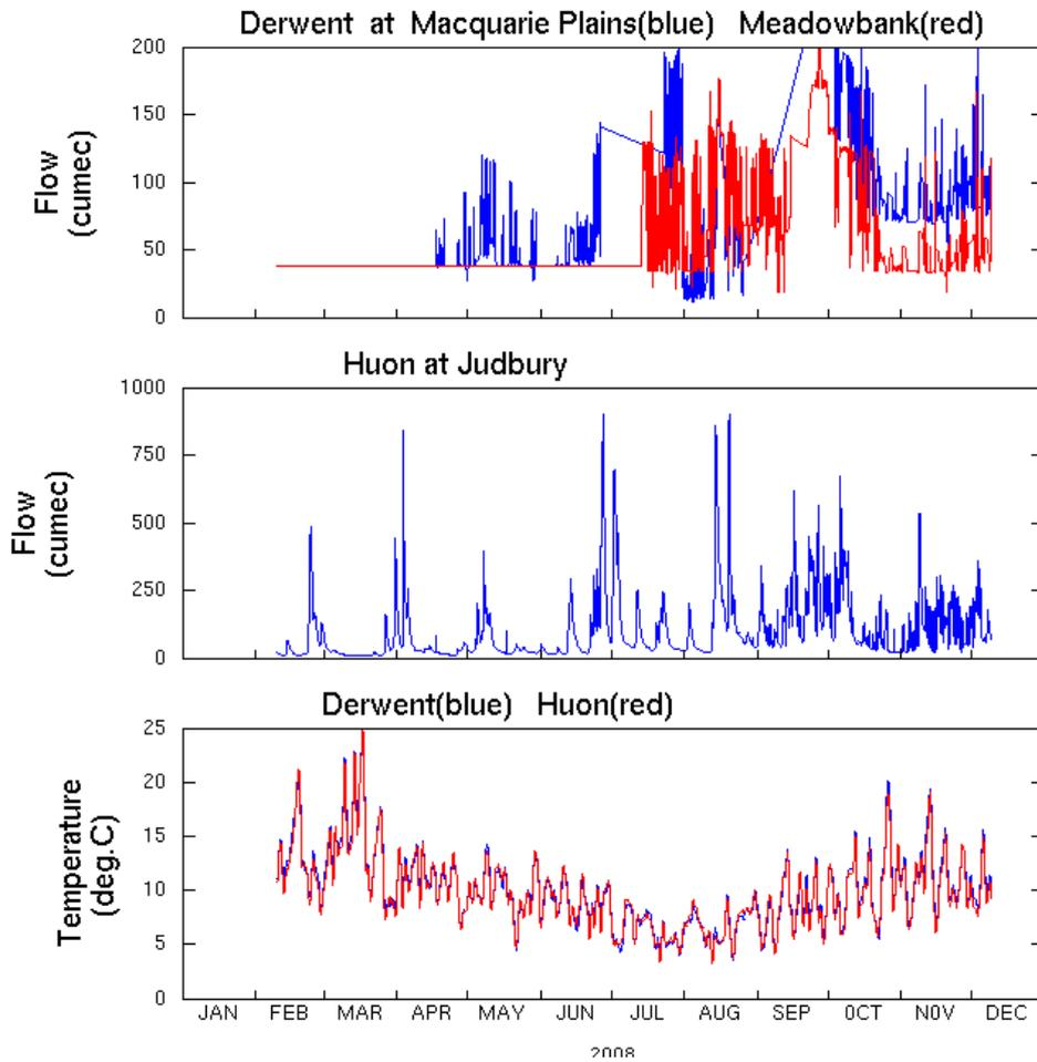
**Figure 2.11. River flow & water temperature for the Derwent & Huon Rivers**
