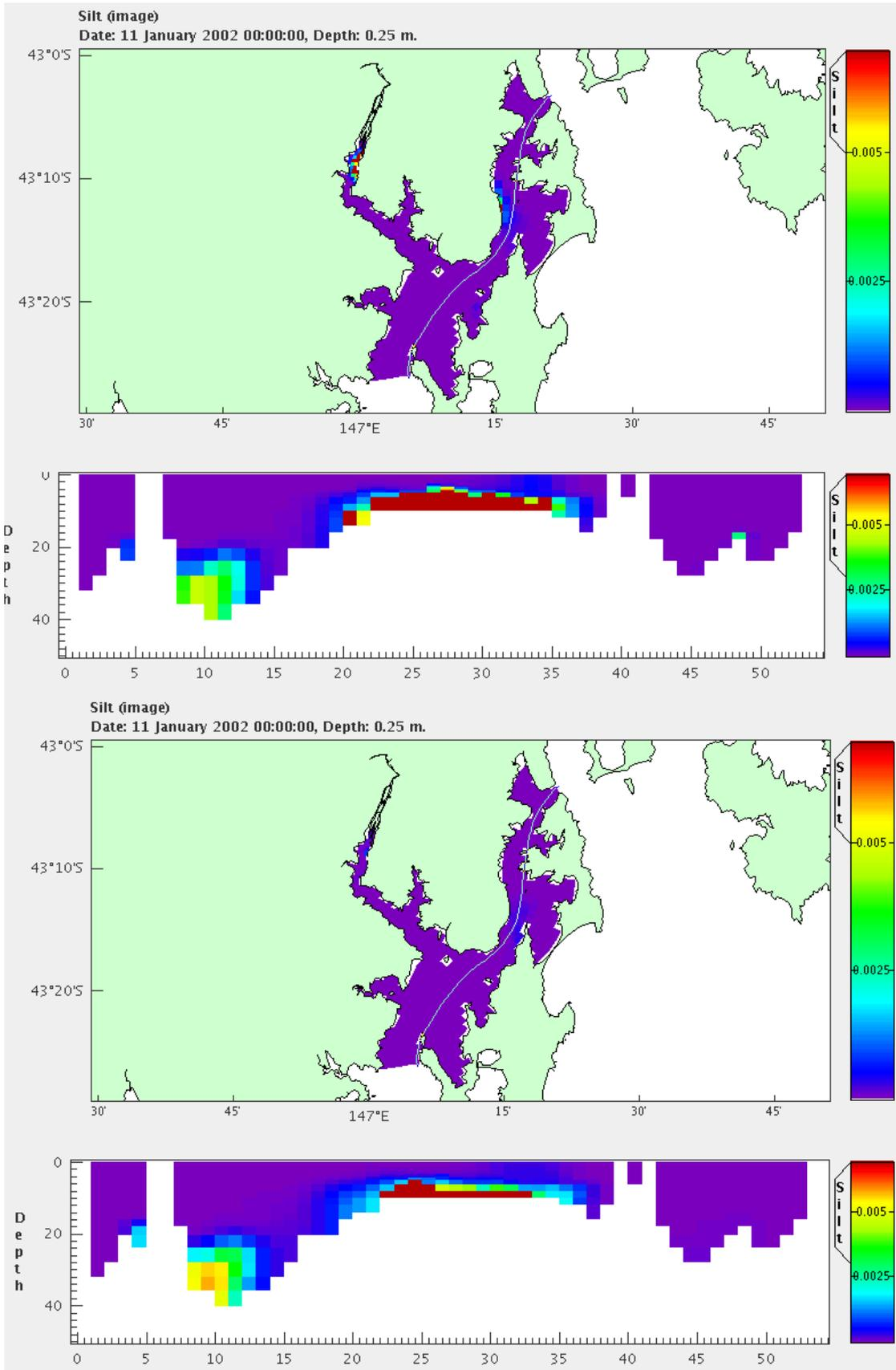
Figure 3.6 Same as above for the silt fraction of sediments.
