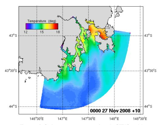
Figure 2.25. Surface temperature output from the SETAS model.
