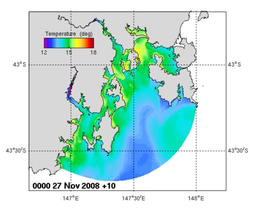
Figure 2.26. Surface temperature output from the STORM model.
