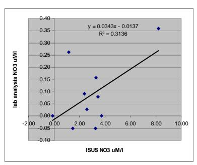
Figure 4.2.7: Comparison of laboratory and ISUS determined nitrate concentration for all samples analyzed. A linear trend line is fitted with R2 value of 0.3.
