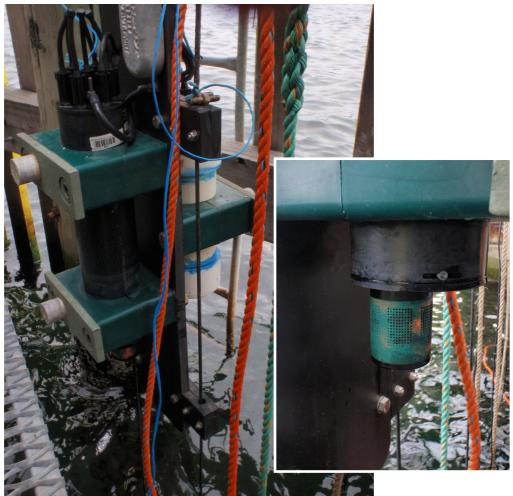
Figure 4.2.1: ISUS deployment on wires under CMAR wharf. Inset image shows copper sensor cover (with fine mesh insert).
