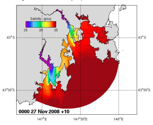
Figure 2.28. Surface salinity output from the STORM model.
