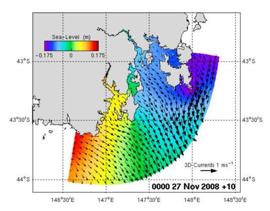
Figure 2.23. Surface elevation and currents from the SETAS model.
