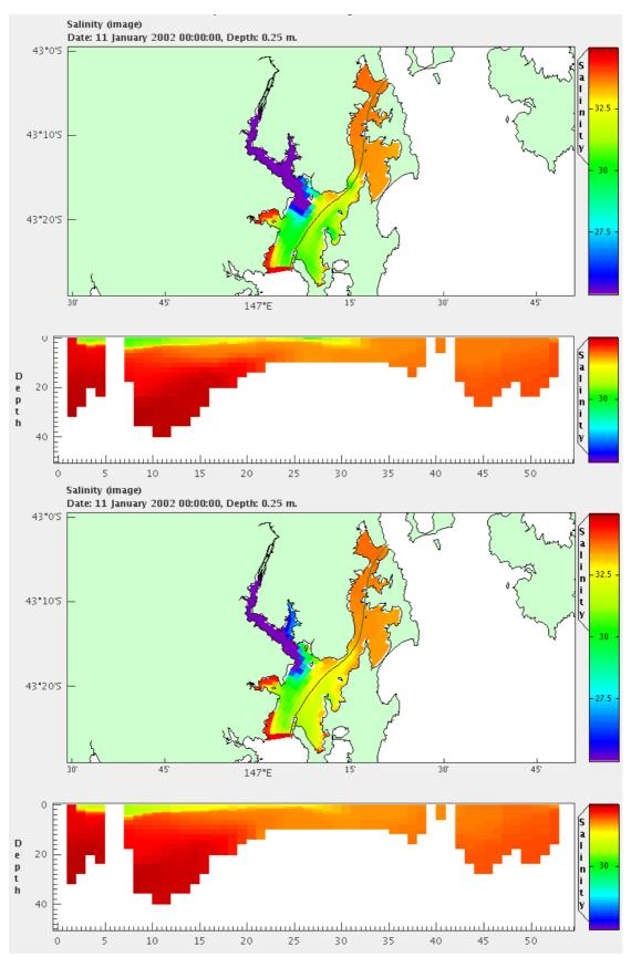
Figure 3.5 Surface and vertical cross-section of salinity simulated with fully coupled (top plots) and decoupled (bottom plots) models. The cross-section line is shown on the surface plot.
