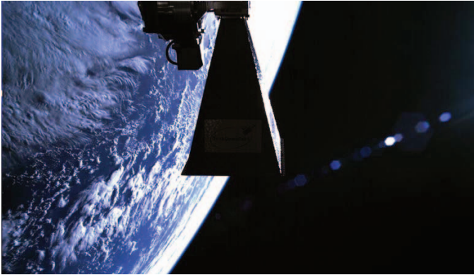
Figure 12: ‘Selfie’ of the SSTL high gain antenna pointing mechanism on board TechDemoSat-1
