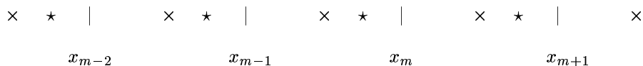
Figure 7: Relative location of unstaggered ( | ) and staggered ( \times ) grid points, and “pivot” points ( \star ).
