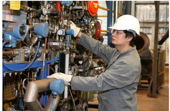
CSIRO pilot-scale pot-grate facility to simulate the sintering process occurring on sinter strands
