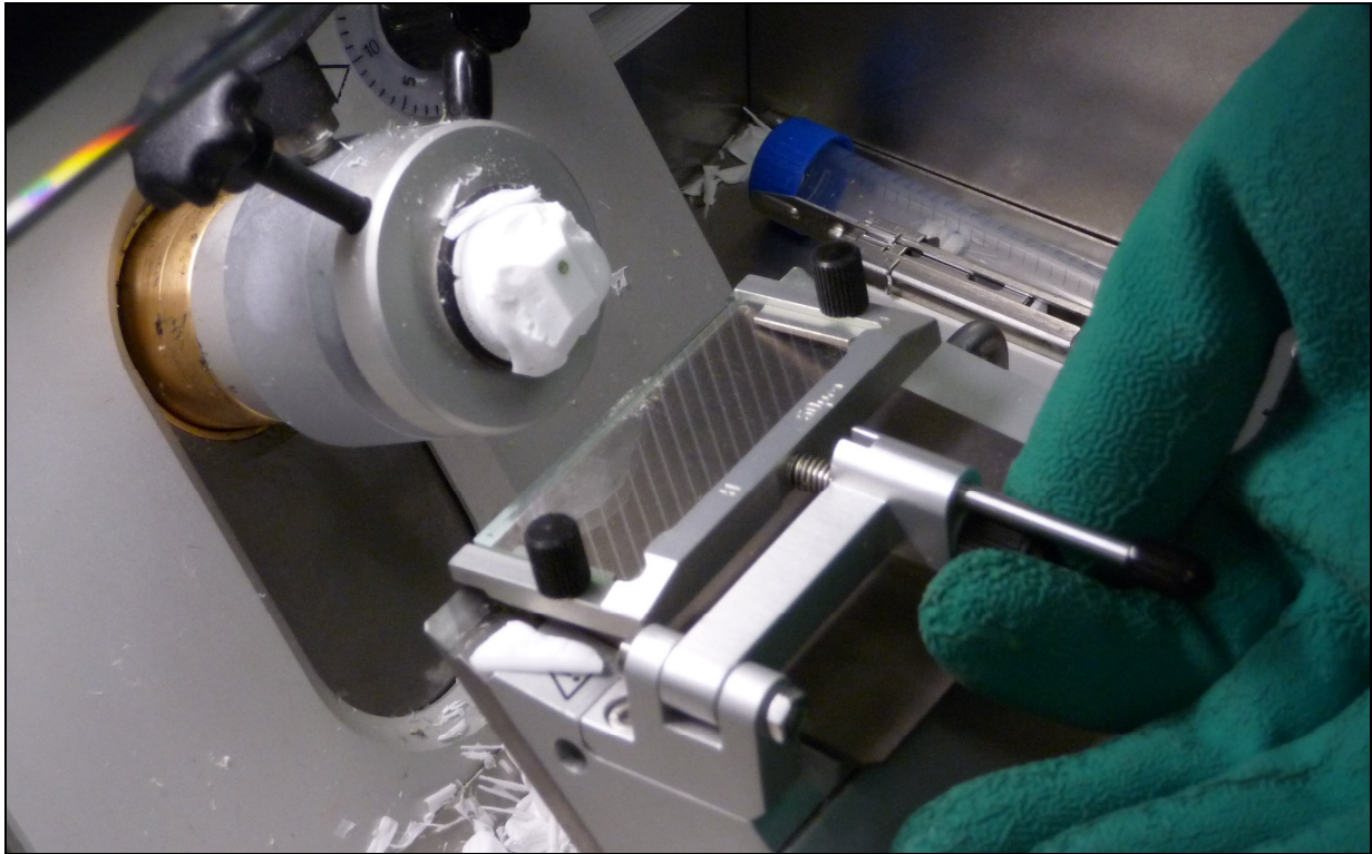
Figure 8. Adjusting the anti-roll plate to catch new sections. The plate should only just hide the blade when viewing from directly above.
