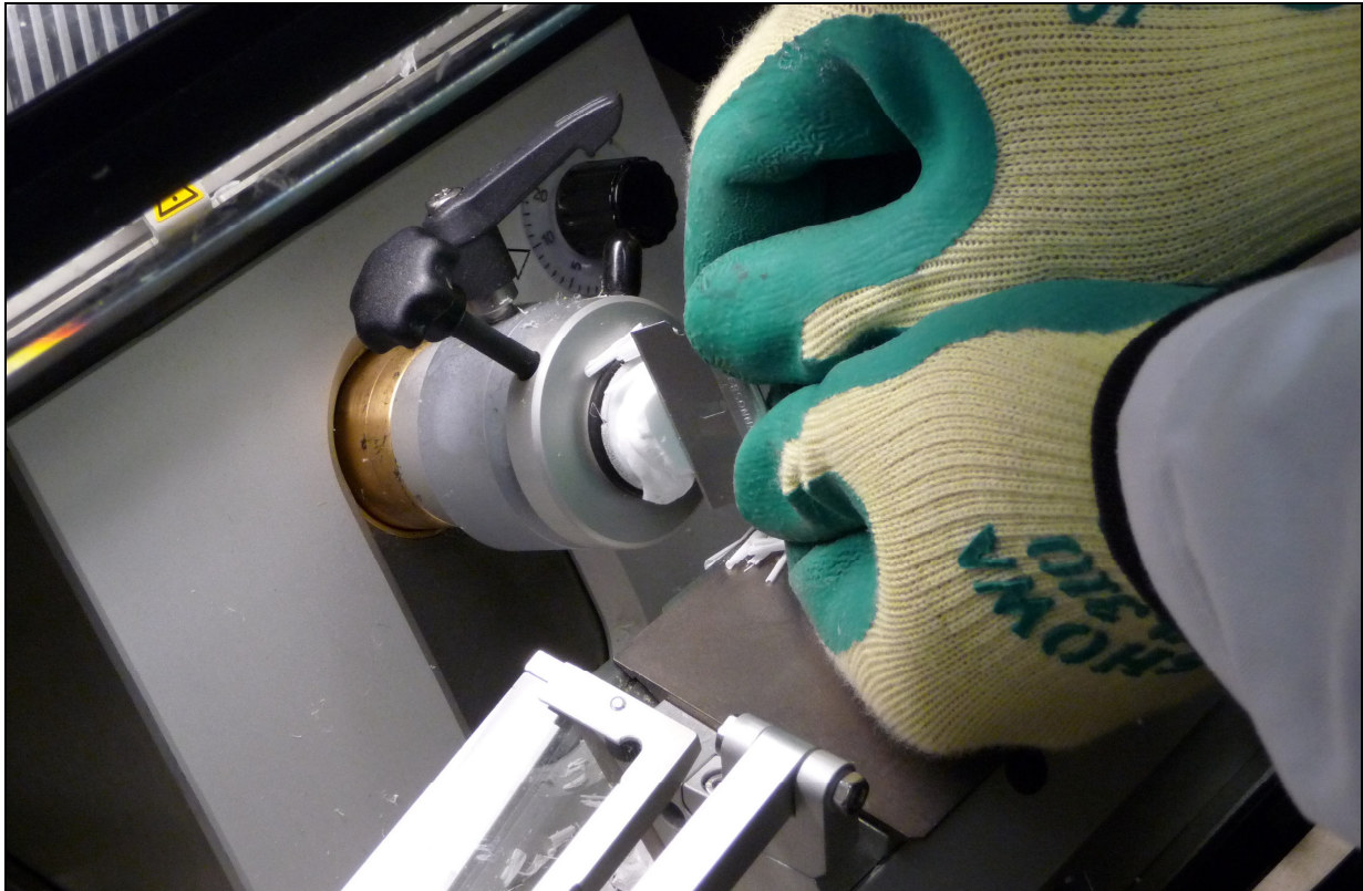
Figure 6. A razor blade is used to remove excess mounting media from the stub.
