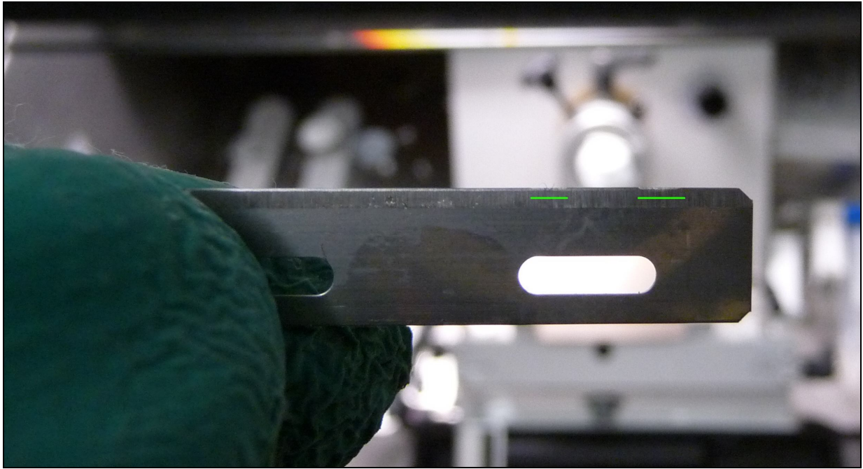
Figure 12. Sectioning blades are quickly blunted. The left side of the blade is unused, while to the right two areas have been highlighted green where the blade is no longer suitable for sectioning.
