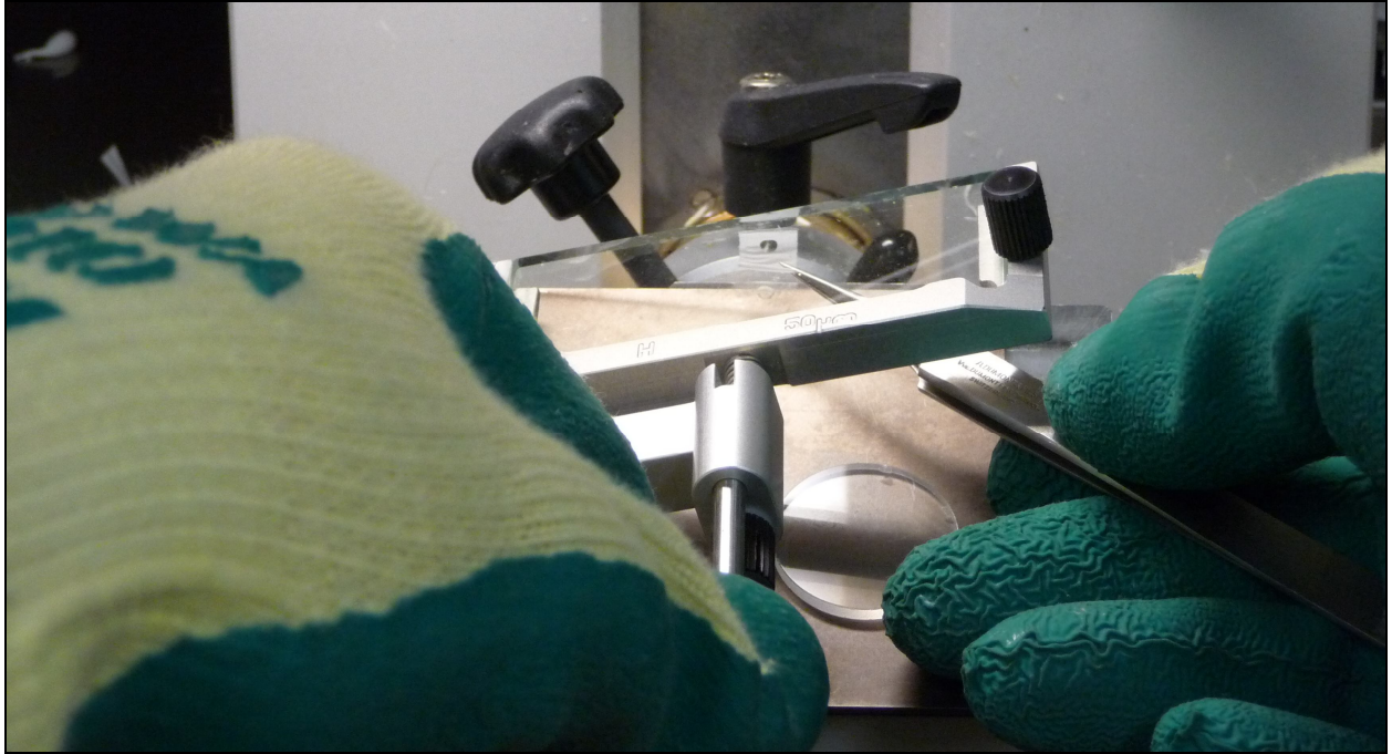
Figure 18. A section is quickly but gently removed from the anti-roll plate with cold forceps, at 45 degrees across the section to help prevent rolling.
