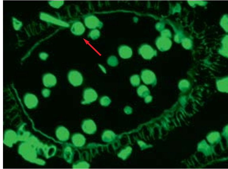
HiLite attached to the observation zoom results in stray light.
