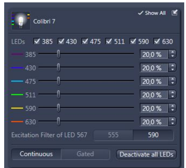
Fig. 17 Control menu for Colibri 7
