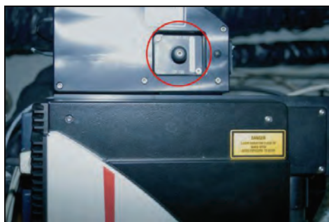
Figure 188: Adaptation at X1 port with SMD filter cube
