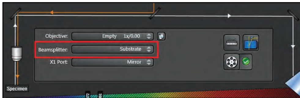
Figure 103: Setting the beam splitter to substrate
