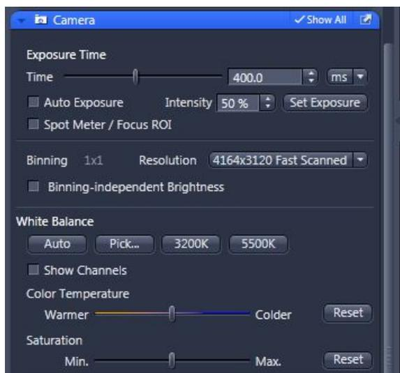
\*Note: It is important to change the intensity of the TL lamp via the software using this slider and **not** the control wheel on the microscope body. Changes using the control wheel are not recorded by the software and it will revert to the original value during image acquisition.
