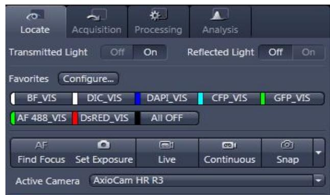
To view an image on the screen, click the live button to display the live feed from the camera and move the eyepiece sliding lever on the microscope turret, detailed in section 1, all the way to the right.
