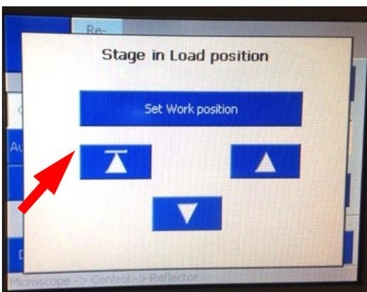
You can also use **Load position** located on the right-hand side of the touch screen to automatically lower the stage to the loading position, shown below.
