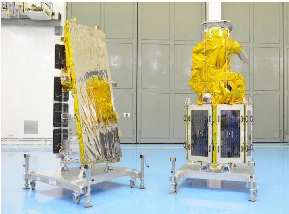
Figure 6-7: NovaSAR-1 and SSTL S1-4, both based on the SSTL-MINI platform (approximately 430 kg launch mass each). Image credit: SSTL.
