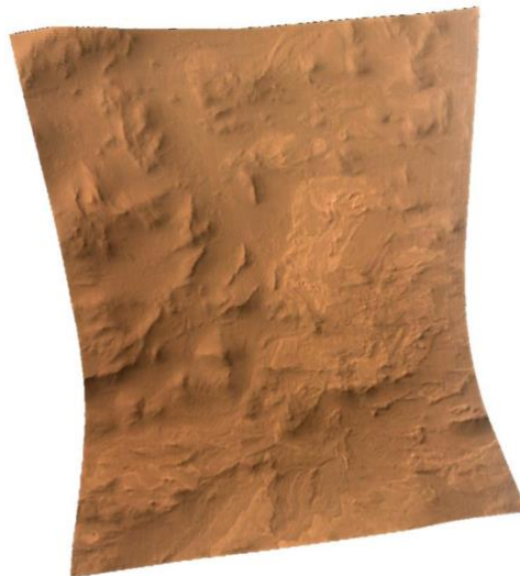
Figure 5-1: Example CRISM image of the Mars surface, showing the characteristic bowtie shape resulting from GMC observations (JPL, 2006).
