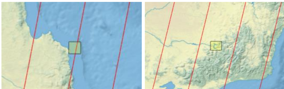
Figure 4-4: Illustration of variance in number of imaging opportunities depending on target location relative to the ground tracks. All passes shown in red correspond to an imaging opportunity for orbit epoch 2024-Jan-01 11:54:40. Left: Lizard Island gives 3 imaging opportunities. Right: Lake Hume gives 4 imaging opportunities.
