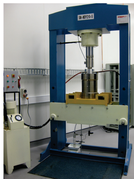
Sand production cell.
