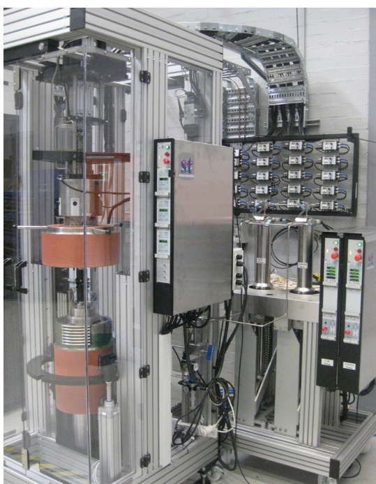
CSIRO's new HPT-Triax Cell is equipped with 20 channels for active ultrasonic and passive micro-seismic monitoring, and can reach pressures up to 150 MPa and temperatures up to 200°C.
