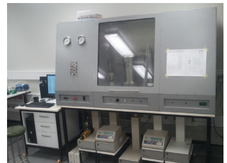
Core flooding rig for unconventional gas studies.
